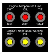
follows: CHT 45°F below redline, OIL 25°F below redline, and TIT 100°F below redline. A two-position toggle switch mounted near the alarm panel will allow you to dim the lights for night operations.
