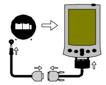
into the data connector on your aircraft instrument panel, and the cradle or travel cable to the Palm handheld.
